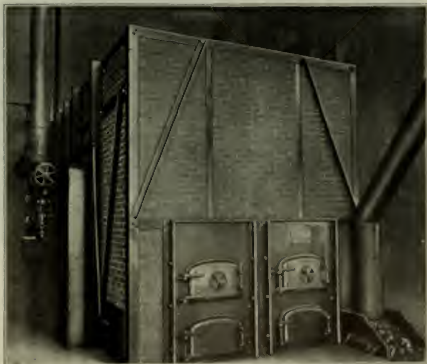
FIG. 8. SEPARATELY FORMED SECTION SUPERHEATER
